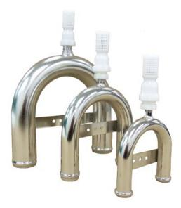
The Vacuum Breaker has a normally closed poppet which keeps vent line fumes from the vessel. The breaker is designed for a corrosion proof service life with a protected air vent. All of the parts exposed to liquid are manufactured from Delrin. The external poppet spring is stainless steel. Liquid never touches the stainless steel spring.
