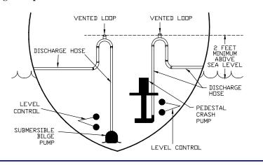
Type 20913 Vented Loops include a sensitive marine vacuum breaker with a stainless steel spring to hold the poppet closed. A vacuum will pull the poppet open, permitting air to go into the system.
